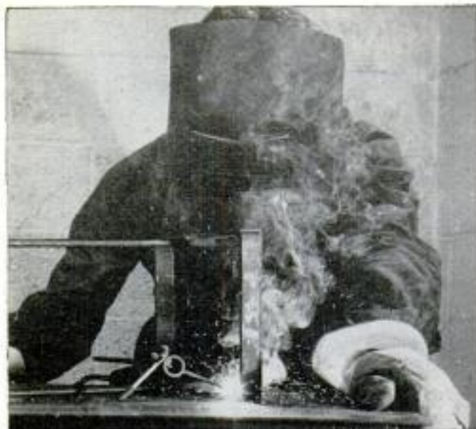
Look... no hands. Just lay the electrode on the work ... Selfweld welds itself.
